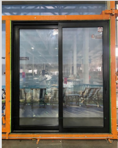
Two side frames and middle are still straight, no adjustments necessary
