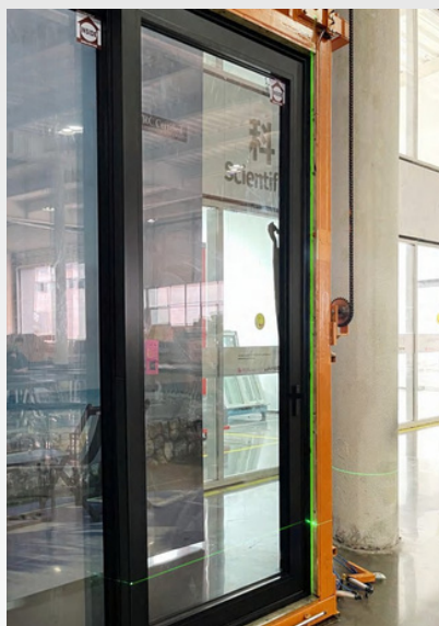
Frame surfaces are still straight, no adjustments necessary
