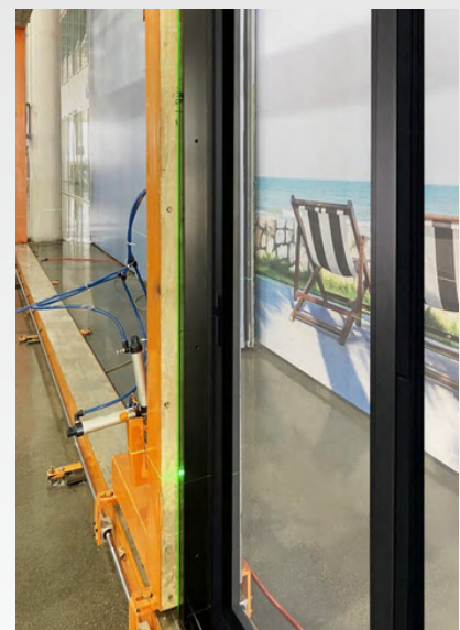
Frame surfaces are still straight, no adjustments necessary
