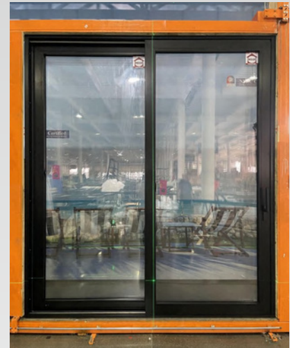
Two side frames and middle are still straight, no adjustments necessary
