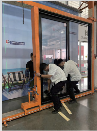
Lower the stationary door panel onto the bottom track
