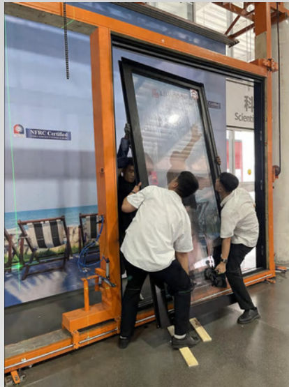
Insert the stationary door panel into the top track
