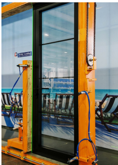
Check four sides in a single plane (Two side frame surfaces straight)
